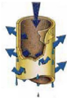
Fig. 1. Coalescing Filter – Used to remove oil and water droplets, particulate matter from compressed air. The liquids drip to the bottom of the filter housing and are automatically emptied by a drain assembly
